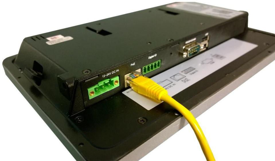
One Ethernet Cable (Cat 5e) connected to a PoE switch will provide data and power
