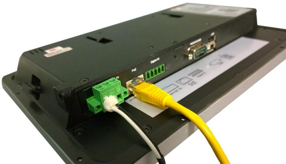
Data provided to the screen via Ethernet cable, Power via supplied power adapter, cable and block.
